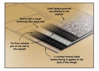
As hail is propelled onto a non-impact resistant shingle, it knocks off granules of the shingle's outer layer—exposing it to UV damage that can degrade the roof and make it vulnerable to leaks.
