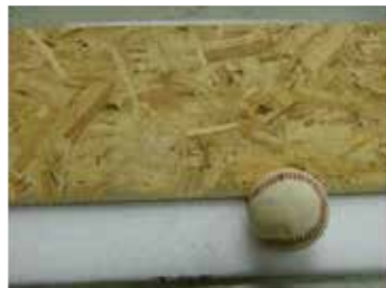
Post-test front (left) and rear (right) photos of LP panel impacted by a baseball in test NASA LVG731
