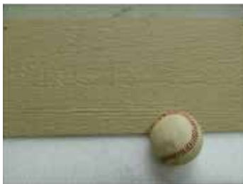
Post-test front (left) and rear (right) photos of LP panel impacted by a baseball in test NASA LVG731
