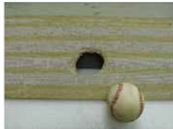
Post-test front (left) and rear (right) photos of fiber cement panel impacted by a baseball in test NASA-LVG733
