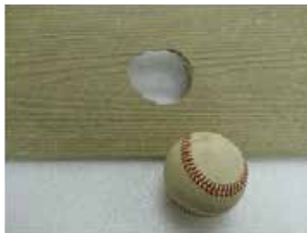
Post-test front (left) and rear (right) photos of fiber cement panel impacted by a baseball in test NASA-LVG733
