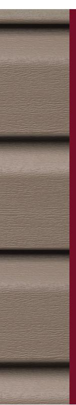
Unlike standard lap siding, which has flat panels that overlap each other at an angle, Dutch Lap has a decorative groove between the laps. This groove improves strength, adds depth and creates wider shadow lines. It's a popular choice for Colonial and Victorian-style homes, as well as hipped-roof styles such as Prairie. Each Double 4.5" DL panel includes two fourand-a-half-inch-wide laps per panel.
